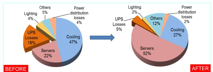
Fig.5. Comparison of the Change in the Proportion of Energy Consumption.
