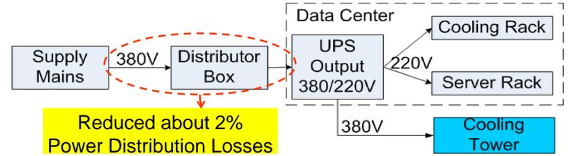
Fig.4. New Voltage Transformation Path.
